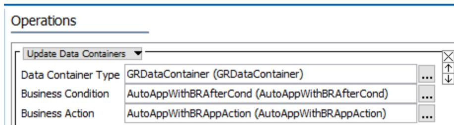
2. In the **Data Container Type** parameter, (optional) click the ellipsis button (...), select the data container type this operation should apply to, and click **Select**.
