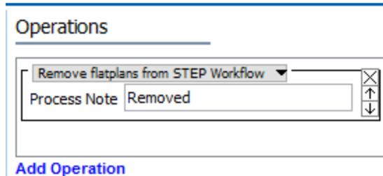
The screenshot shows a configuration window titled "Operations". Inside, there is a dropdown menu currently displaying "Remove flatplans from STEP Workflow". Below the dropdown is a text input field labeled "Process Note" which contains the word "Removed". To the right of the input field are three small icons: a close button (X), an up arrow, and a down arrow. Below the entire configuration area is a blue button labeled "Add Operation".
